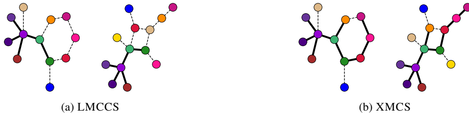
Figure 3: Example graph pairs with node colors indicating the proposed alignments by our models LMCCS and XMCS, for the MCEC setup. In Panel (a), LMCCS proposes an alignment which results in an MCEC score of 6. In Panel (b), XMCS proposes an alignment on the same query-corpus pair, which results in an MCEC score of 10. The connected nodes in both cases are identified by thick black edges.
